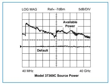
In application, find the Available Power for the instrument being used in the measurement. A comparison between P STOP and the Available Power indicates whether enough power is available for the measurement.
