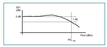
This gain compression curve has been labeled to show the output 1 dB compression point.
