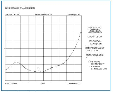
Figure 3. Group delay of an amplifier
