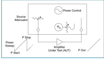
Figure 4. Block diagram of test environment
